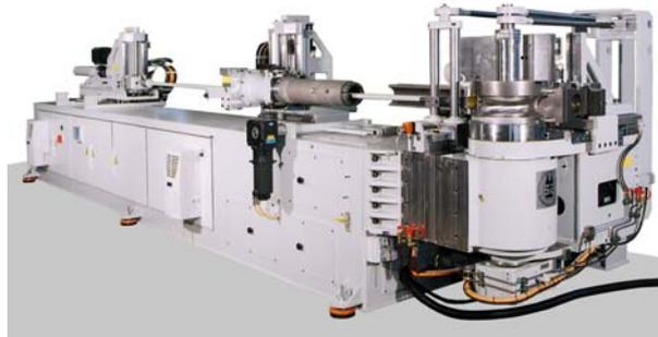
Maximum energy efficiency with top performance: The fully electric CNC 100 E TB MR tube bending machine is suitable for tubes with diameters from 25 to 114.3 mm.
